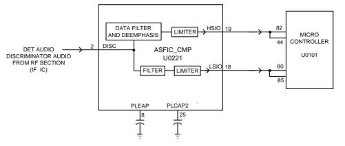
Figure 2-6. Receive Signalling Paths
