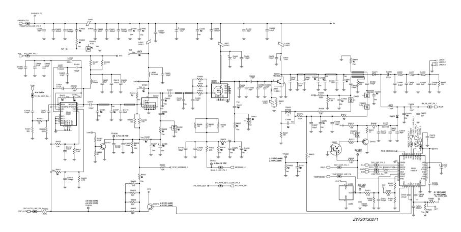
Figure 4-18. UHF (403-470MHz) Power Amplifier Schematic Diagram
