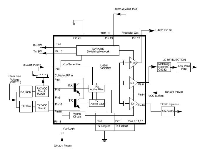
Figure 2-10. UHF VCO Block Diagram
