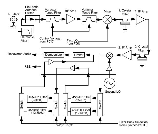
Figure 2-7. UHF Receiver Block Diagram
