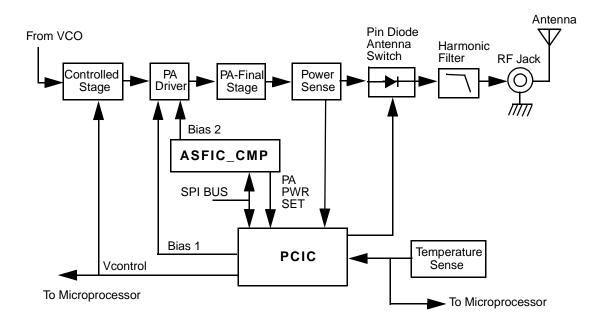
Figure 2-8. UHF Transmitter Block Diagram
