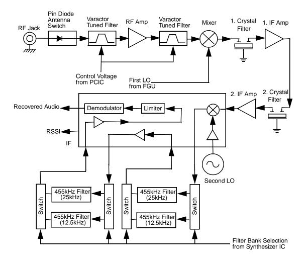
Figure 2-11. VHF Receiver Block Diagram
