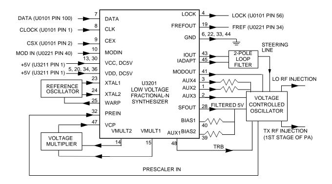
Figure 2-13. VHF Synthesizer Block Diagram
