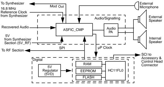
Figure 2-1. Controller Block Diagram
