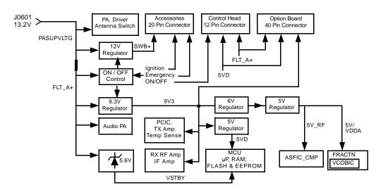
Figure 2-2. DC Power Distribution Block Diagram
