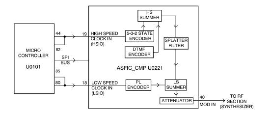
Figure 2-4. Transmit Signalling Paths
