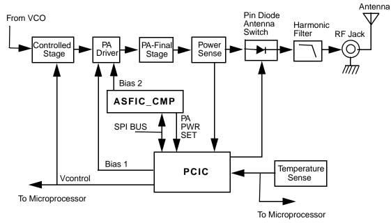
Figure 2-12. VHF Transmitter Block Diagram
