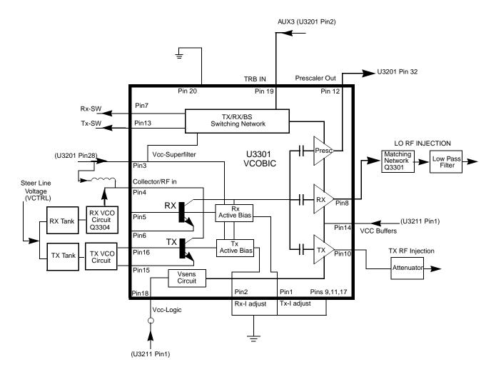
Figure 2-14. VHF VCO Block Diagram
