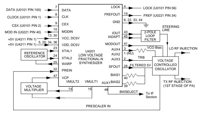
Figure 2-9. UHF Synthesizer Block Diagram
